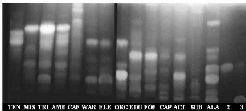
Figure 3. Pattern of hydroethanolic extracts from Passiflora species. Chromatographic system: Si gel GF 254 , CHCl 3 :EtOH:AcOH (60:40:5, v/v), anisaldehyde-H 2 SO 4 then heating (100°C)/UV 366 . To sample codes see materials and methods. Reference: 3-O-β-D-glicopiranosil-1 → 2-β-D-glicopiranosil-oleanolic acid ( 2 ) and quadranguloside ( 3 ).
