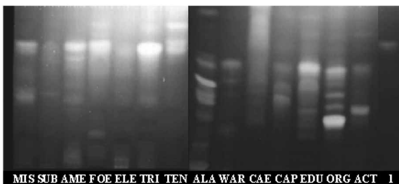
Figure 2. Pattern of hydroethanolic extracts from Passiflora species. Chromatographic system: Si gel GF 254 , AcOEt:acetone:AcOH:H 2 O (60:20:10:10, v/v), anisaldehyde-H 2 SO 4 then heating (100°C)/UV 366 . To sample codes see materials and methods. Reference: vitexin (1).
